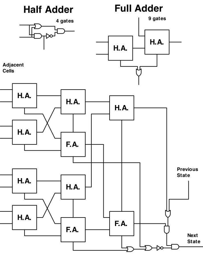
7 half adders (28 gates), 3 full adders (27 gates), 6 other gates, TOTAL: 61 gates If XOR were allowed, subtract 26 gates. If NOR were allowed, subtract 1 gate.
